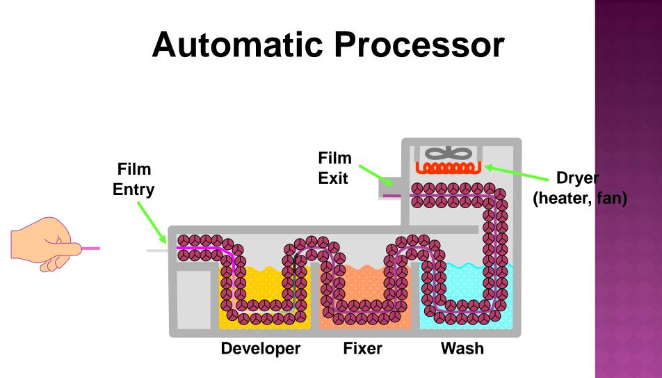
The rollers "squeegees" the excess chemicals off of the film as it exits each solution; no rinse is needed between the developer and fixer.
